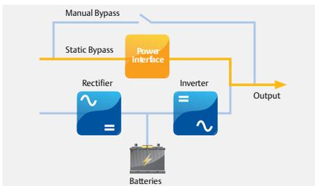
**Maximum Energy Saving (VFD)** detects when conditioning is not required and allows the energy flow to pass through the bypass line.
