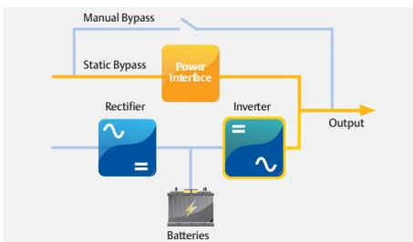
**High Efficiency & Power Conditioning (VI)** compensates the load THDi, PF and main sags and swells.
