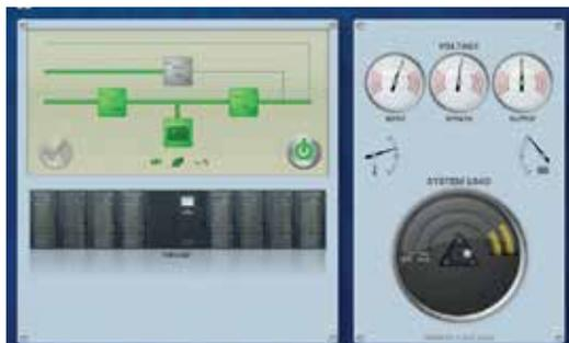
System status, measurements and single-line diagram.
